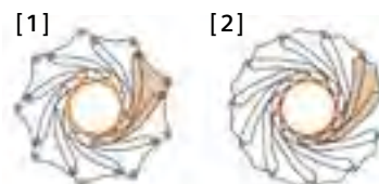
[1] Conventional aperture [2] Circular aperture
